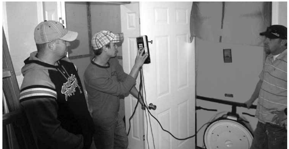
Student Travis Skelton sets up a blower door, which puts negative pressure on the house to detect air leaks. At left is student Matt Ferguson .
